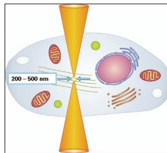
Left: Linear absorption – constant absorption coefficient ( $\mu_a$ ); non linear absorption -  $\mu_a$  depends on intensity of light (fs-laser pulses) and enables a very small focal volume (< 1 $\mu$ m in diameter).
