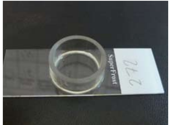
Fig. 1: Microscope slide with chamber to keep tissue in Ringer solution during sectioning
